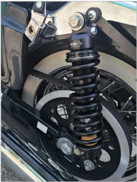
TM1 "C65" spring preload ring tool included
